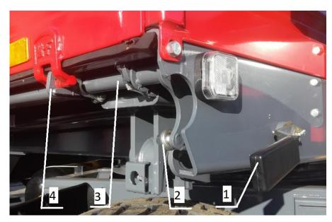
**Fig. 19.** The locks on the sideboards of the load-carrying body: 1 – central lever of the bottom locks, 2 – lock adjustment mechanism, 3 – central lock shaft, 4 – lock
